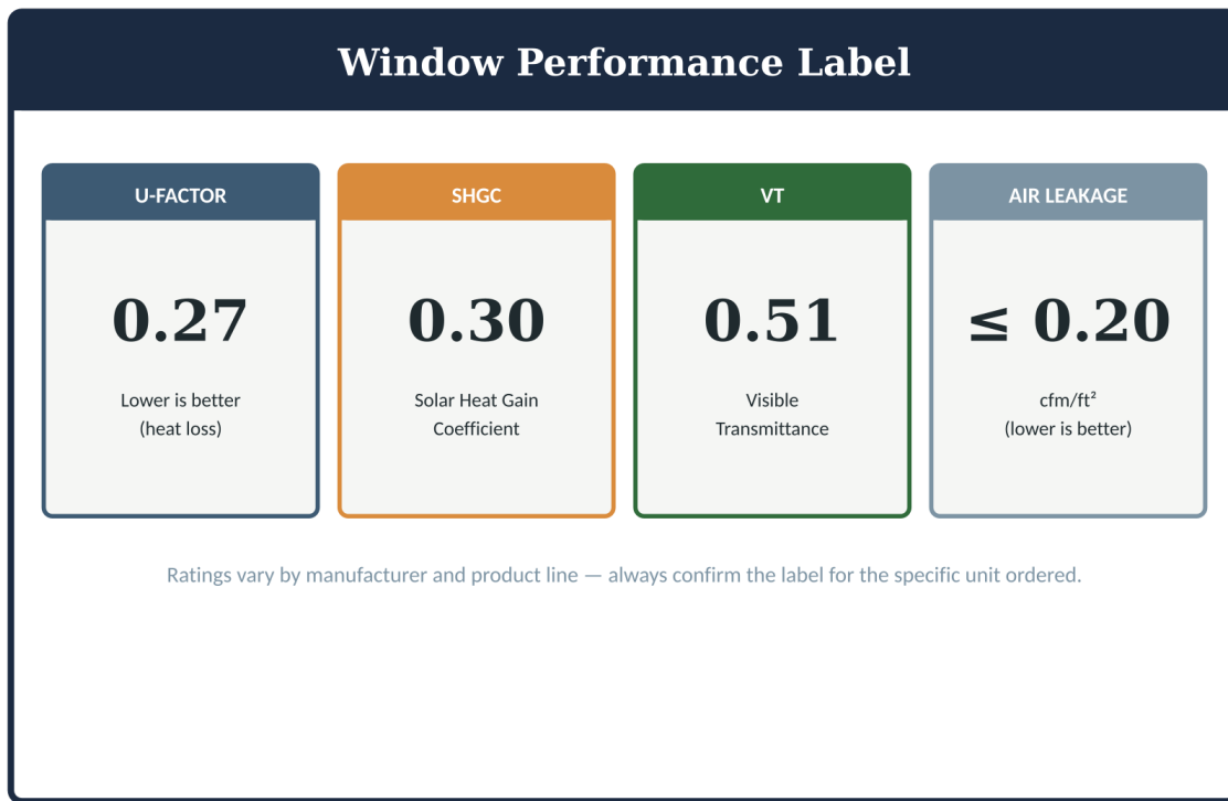
Figure 1 — A typical window performance label and what each rating means.
